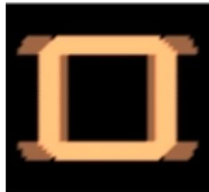
**Figure 13.** A square-ring annulus shape for off-axis illumination. This source is optimized for  $k_1$  near 0.40. Maximum overlap of diffraction orders is achieved, which is superior to circular-ring annular illumination.
