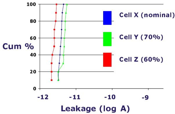
Figure 24: Poly to poly isolation versus cell type.
