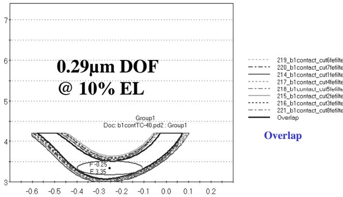
Figure 18: Common process window for 40nm upsized contacts.
