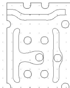
Figure 22: Optimal poly and contact resist image overlay
