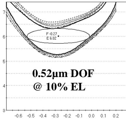
Figure 19: Common process window for un-biased contacts.
