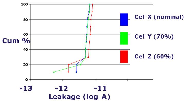
Figure 26: Metal-1 to metal-1 isolation versus bitcell type
