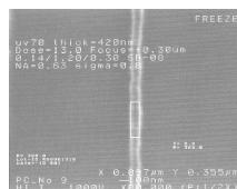
Figure 4. Top down SEMs of 0.14 \mu m lines in a pitch of 1.34 \mu m. The exposure latitude is 7.6% for 0.6 \mu m depth of focus requirement.
