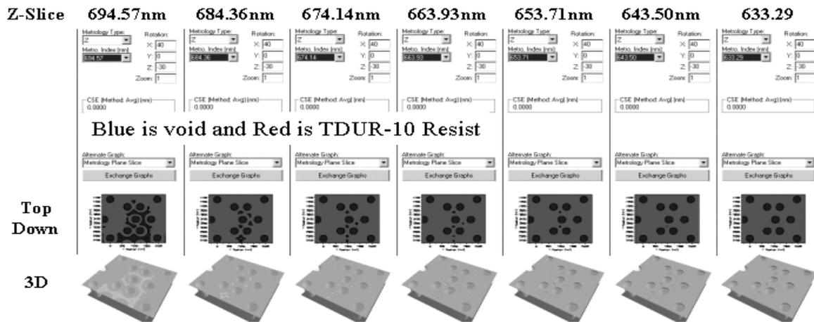
Figure 20: Resist film thickness z-slices of contacts that were 75% overexposed from nominal.
