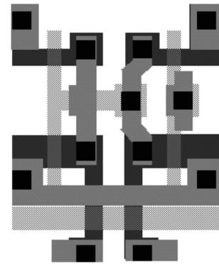
Figure 4: SRAM bitcell layout. Circles indicate critical points for OPC to retain cell margin.
