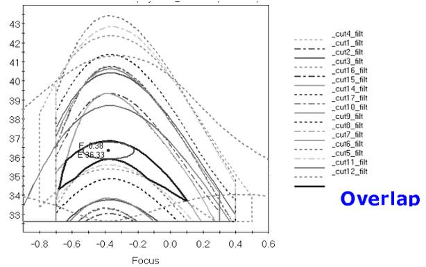
Figure 11 Focus/exposure window after first poly correction iteration.
