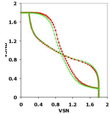
Figure 27: Butterfly curves of scaled area bitcells indicated slight asymmetry derived from misalignment.
