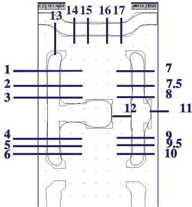
Figure 8: Sample cuts for each transistor positioned at edges & middle of device. Inter-feature spacings also show window for all uncorrected poly sample cuts.
