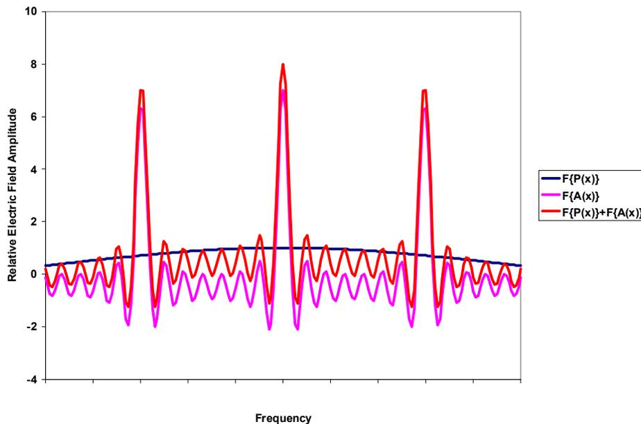
**Figure 8** Fourier transforms of a binary mask with 130nm primary and seven pairs of 65nm assist features with  $Dx$  of 297.5nm.  $F\{P(x)\}$  is the transform of the primary.  $F\{A(x)\}$  is the transform of the seven pairs of assist features.  $F\{P(x)\} + F\{A(x)\}$  is the sum of all transforms. The amplitude is relative to  $F\{P(x)\}$ . Frequency is  $\pm 2NA$ .
