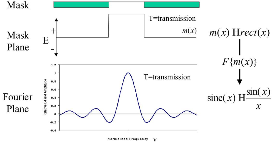
**Figure 1** Cross section of mask with an isolated space. The electric field at the mask plane forms a  $\text{rect}(x)$ . At the Fourier plane, the diffraction pattern is described by the Fourier transform of the  $\text{rect}(x)$  which is  $F\{m(x)\} = \text{sinc}(x)$  function.
